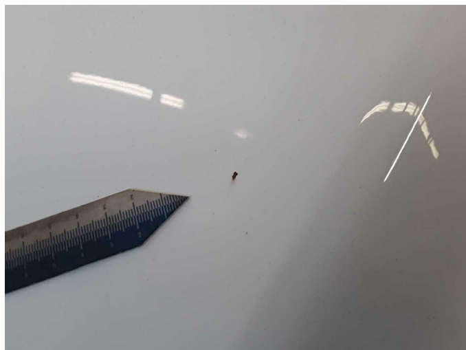
Damage 8: Bonnet: Bonnet - Corrosion - Repair and paint
