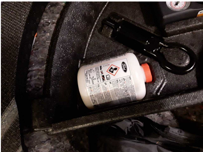
Damage 1: Equipment: Tirefit filler - Expired - Replace
