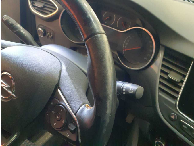
Damage 8: Steering system: Steering wheel sheath (Leder) - Worn - Replace
