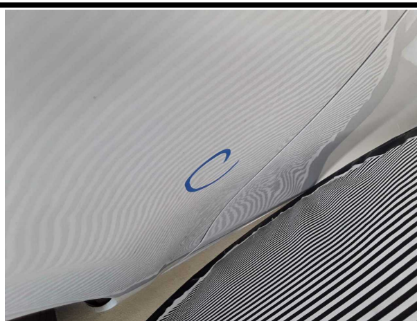
Damage #7: Side panel - rear right side: Side panel - dent(s) - Smooth repair work
