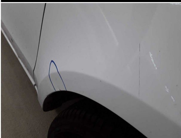
Damage #9: Mudguard - right side: Mudguard - right side - Dent / paintcoat damage - Repair and paint
