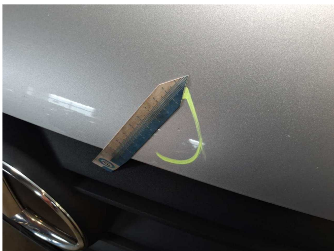
Damage 6: Bonnet: Bonnet - Stone chips - Paint
