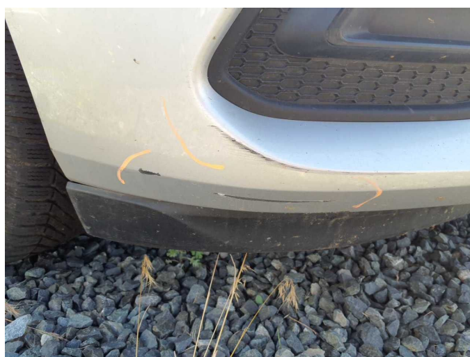
Damage 14: Front bumper: Front bumper - Scratch(es) - Paint
