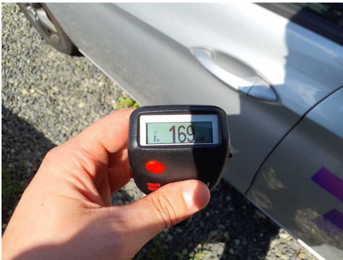
Repainting 4: Door - front left side
