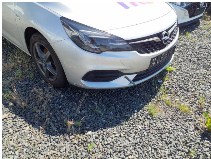
Damage 14: Front bumper: Front bumper - Scratch(es) - Paint
