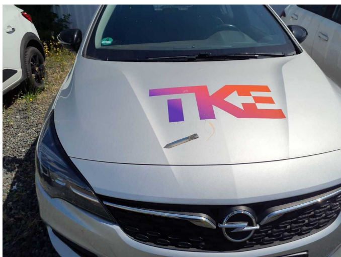
Damage 20: Bonnet: Bonnet - Dent / paintcoat damage - Repair and paint
