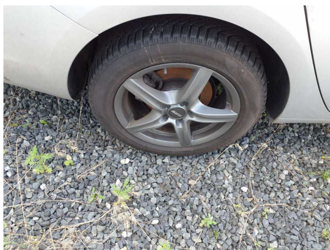
Damage 11: Braking system: Brake discs and pads - rear (Tragbild mangelhaft, Rost) - Corrosion - Replace
