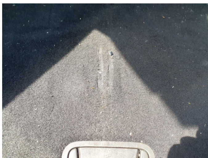
Damage 4: Interior: Cargo area floor - Scratch(es) - Loss in value
