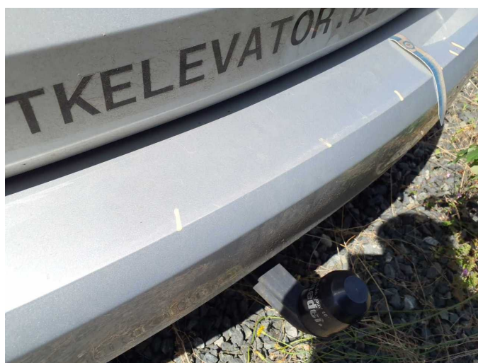
Damage 17: Rear bumper: Rear bumper - Dent / paintcoat damage - Repair and paint
