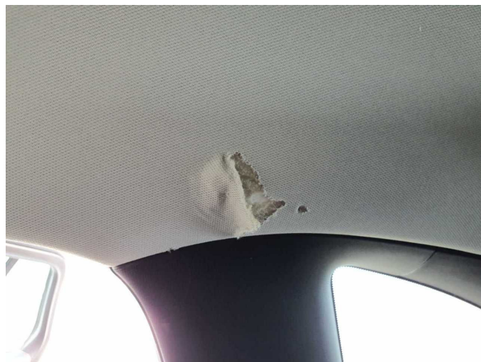
Damage 18: Trim / covers: Roof lining - Broken / torn - Replace
