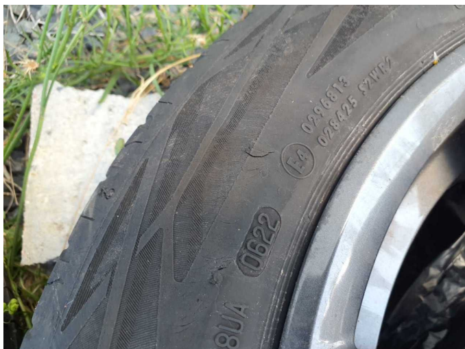
Damage 5: 2nd wheel set: 1 tyre - Broken / torn - Replace
