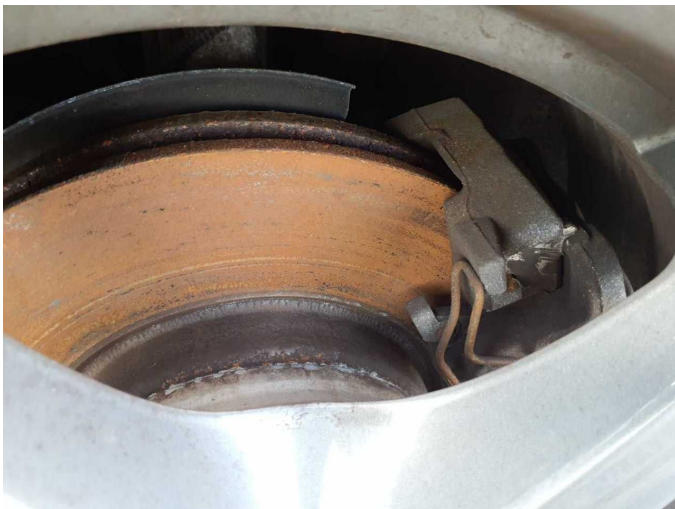
Damage 12: Braking system: Brake discs and brake pads - front (Tragbild mangelhaft, Rost) - Corrosion - Replace
