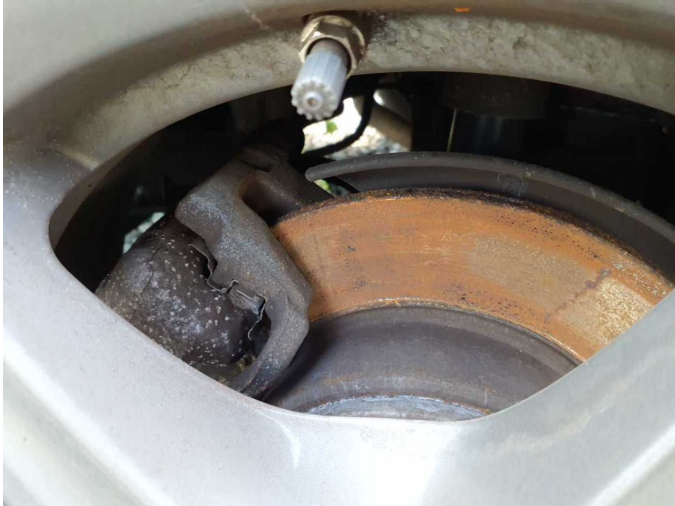
Damage 11: Braking system: Brake discs and pads - rear (Tragbild mangelhaft, Rost) - Corrosion - Replace
