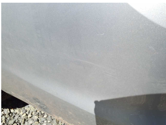
Damage 17: Rear bumper: Rear bumper - Dent / paintcoat damage - Repair and paint
