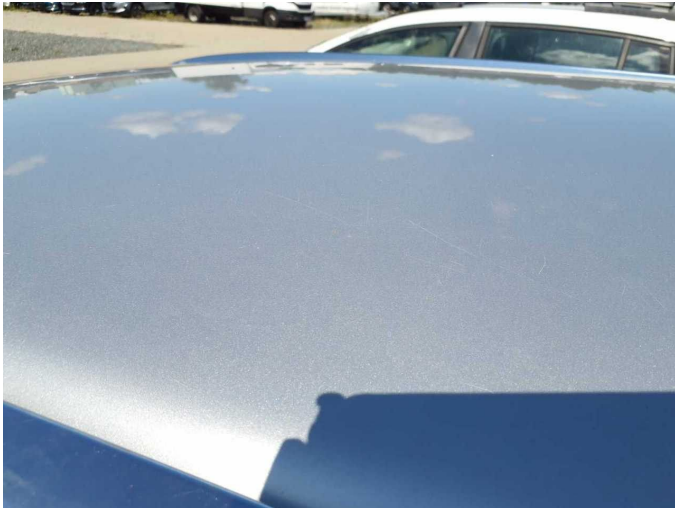
Damage 22: Roof: Roof - Scratch(es) - Paint
