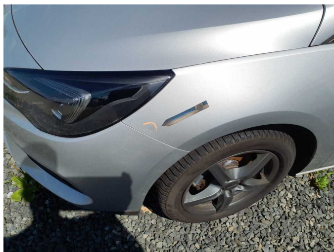
Damage 9: Mudguard - left side: Mudguard - left side - Dent / paintcoat damage - Smart repair
