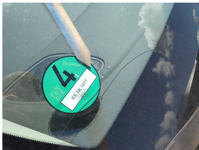
Damage 19: Vehicle glazing: Windscreen - Broken / torn - Replace
