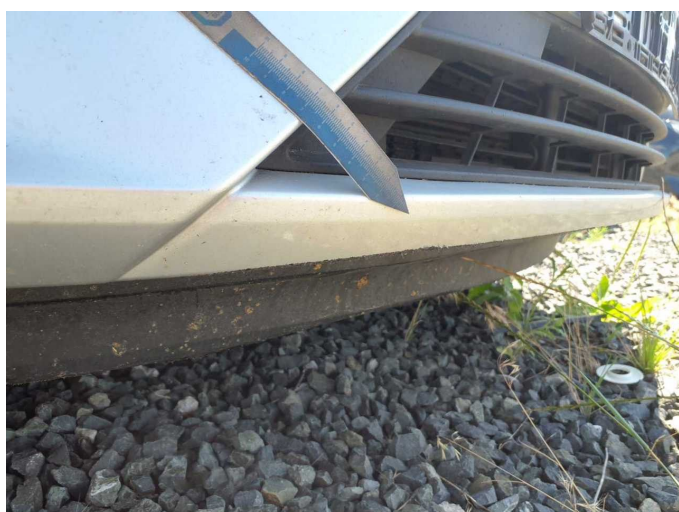
Damage 14: Front bumper: Front bumper - Scratch(es) - Paint
