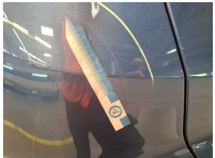
Damage 9: Rear bumper: Rear bumper - Scratch(es) - Paint
