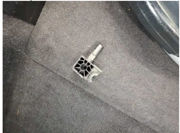
Damage #4: Interior: Rear shelf - Broken / torn - Replace
