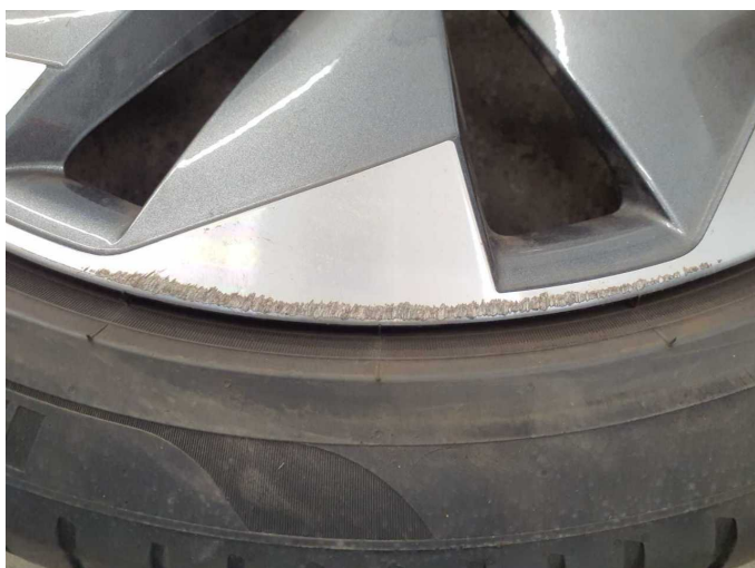
Damage 8: 2nd wheel set: 1 alloy rim (Materialabtrag) - Scratched - Replace
