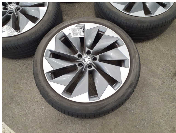
Damage 10: 2nd wheel set: 1 alloy rim (Materialabtrag) - Scratched - Replace
