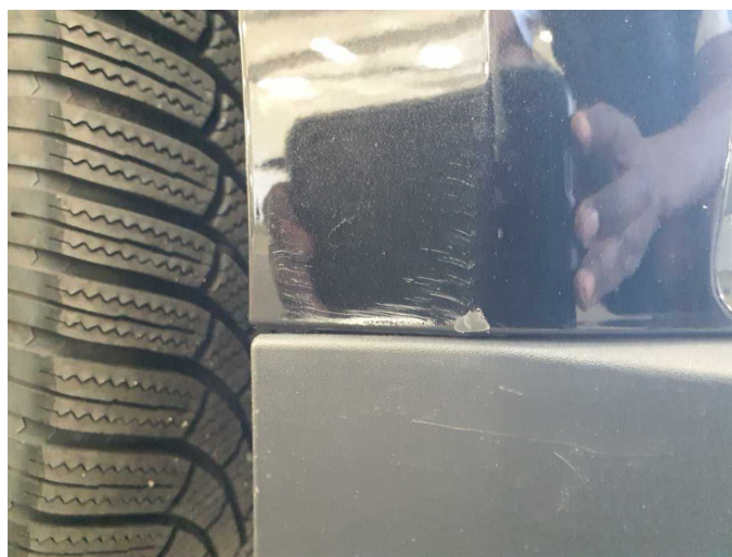
Damage 7: Front bumper: Front bumper - Scratch(es) - Paint
