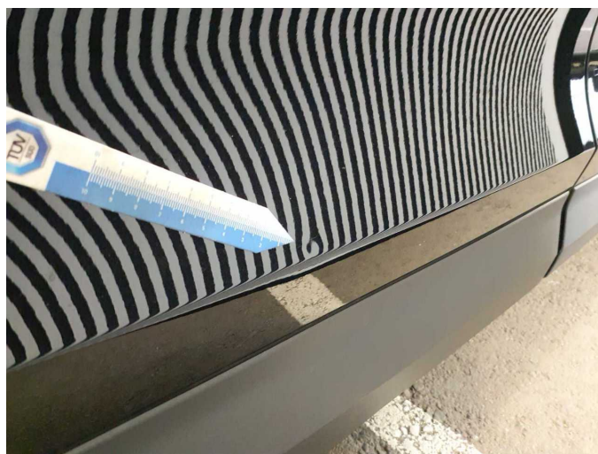
Damage 4: Door - rear right side: Door - dent(s) - Smart repair
