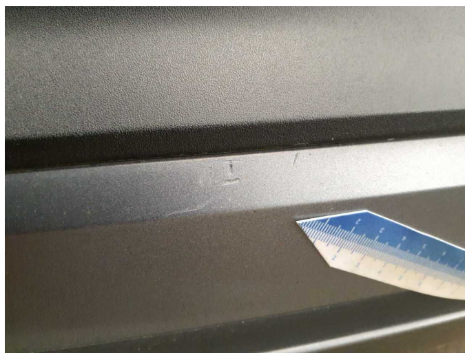
Damage 5: Rear bumper: Spoiler - Scratch(es) - Loss in value
