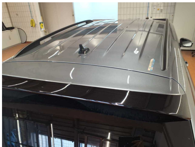
Damage 7: Roof: Roof (+ Steinschlag) - dent(s) - Repair and paint
