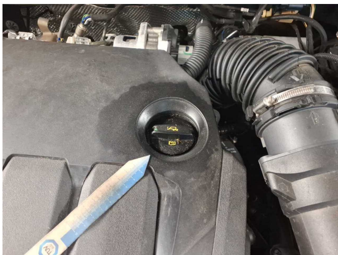
Damage 2: Engine: Engine - Leaking - Perform diagnosis
