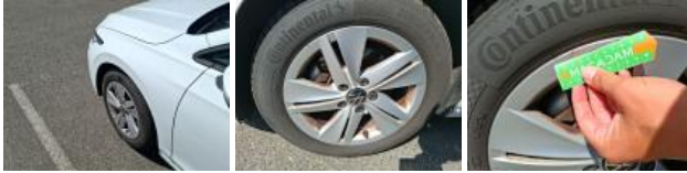
Wing FL, Stone chip(s), Acceptable
