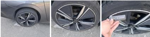
Tyre RR, Tear, Replace
