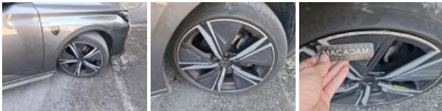
Tyre FR, Out of tolerance, Replace
