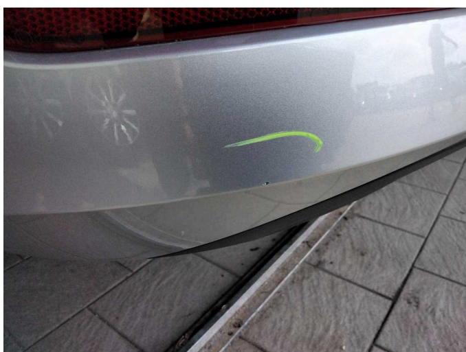
Damage 8: Rear bumper: Rear bumper - Scratch(es) - Paint
