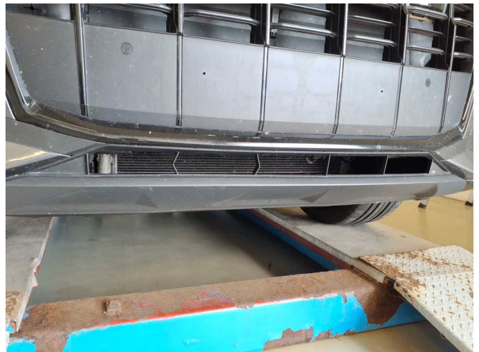
Damage 1: Front bumper: Air-inlet grille - Deformed - Replace
