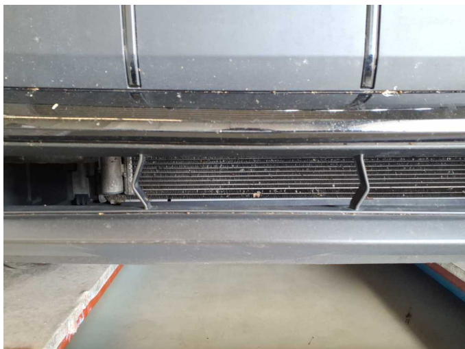
Damage 1: Front bumper: Air-inlet grille - Deformed - Replace
