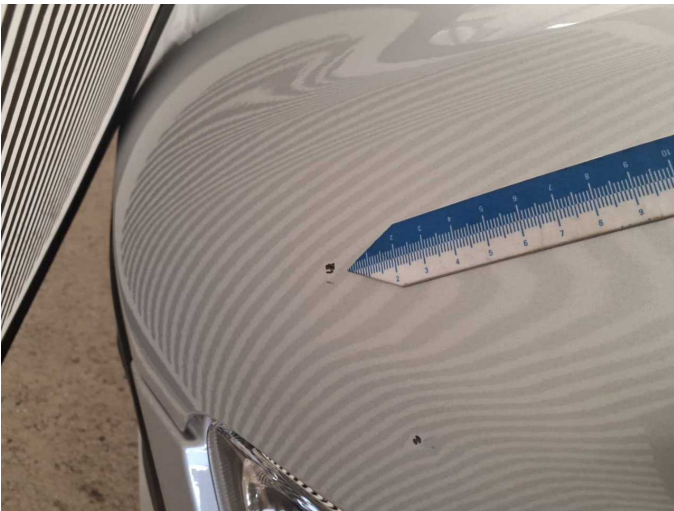
Damage 2: Bonnet: Bonnet - Dent / paintcoat damage - Repair and paint
