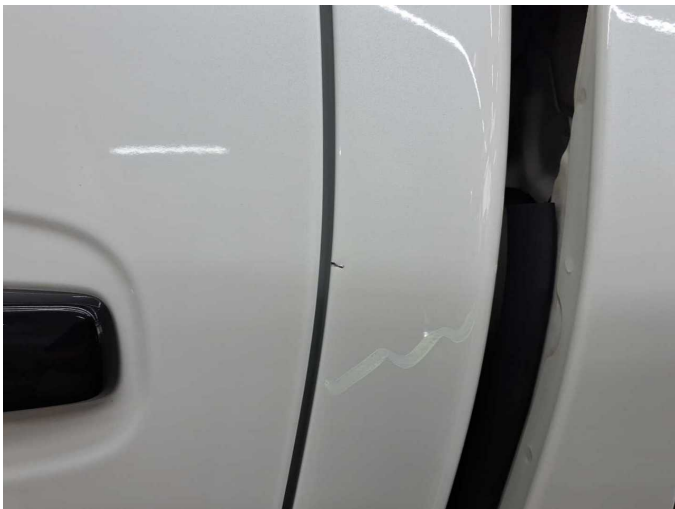
Damage 1: Body: C-pillar - left side - Scratch(es) - Smart repair
