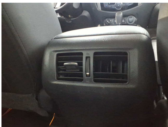
Damage 3: Instrument panel: Air nozzle - centre (Hinten) - Broken / torn - Replace
