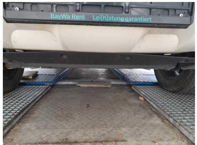
Damage 2: Front bumper: Spoiler - Loose - Replace
