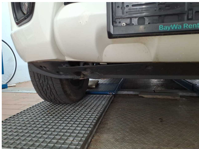
Damage 2: Front bumper: Spoiler - Loose - Replace
