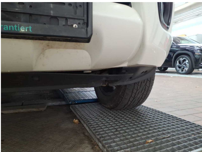
Damage 2: Front bumper: Spoiler - Loose - Replace
