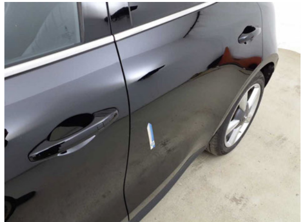
Beschädigung #2: Tür hinten links: Tür - Delle(n) - Smart Repair
