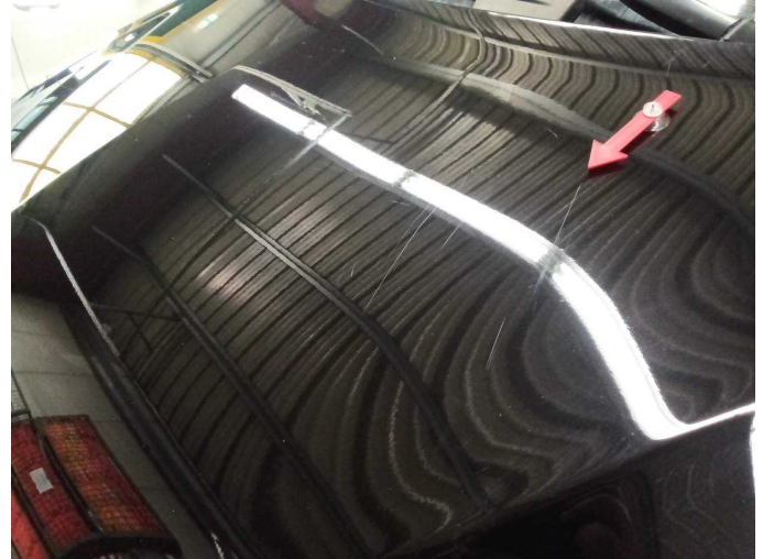
Damage 5: Bonnet: Bonnet - Scratch(es) - Paint
