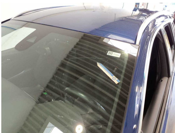
Damage 13: Vehicle glazing: Windscreen - Broken / torn - Replace
