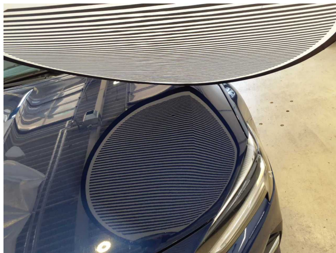
Damage 17: Body: Body - Damage by hail - Repair
