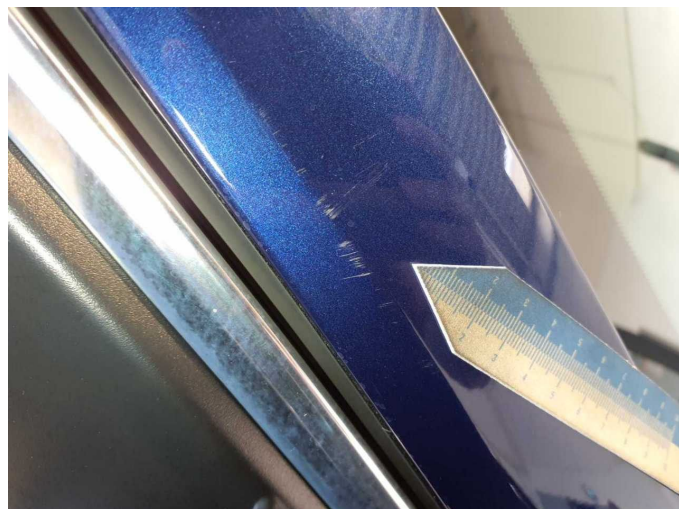
Damage 6: Body: A-pillar - right side - Scratch(es) - Smart repair
