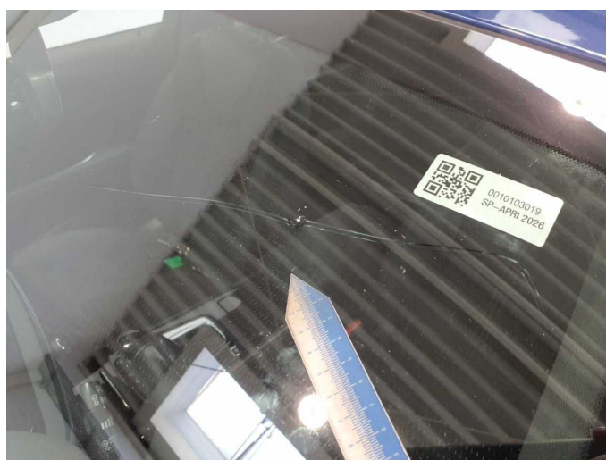
Damage 13: Vehicle glazing: Windscreen - Broken / torn - Replace
