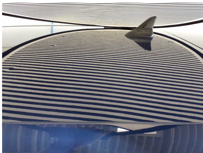
Damage 17: Body: Body - Damage by hail - Repair
