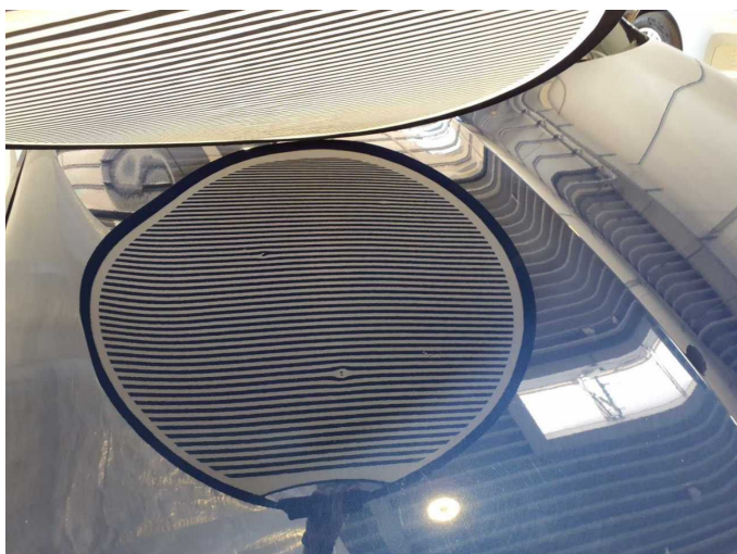
Damage 17: Body: Body - Damage by hail - Repair
