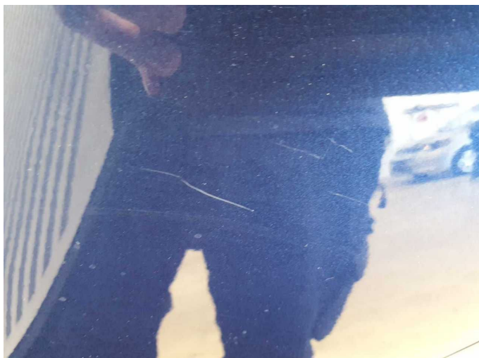
Damage 12: Side panel - rear left side: Side panel - Dent / paintcoat damage - Paint
