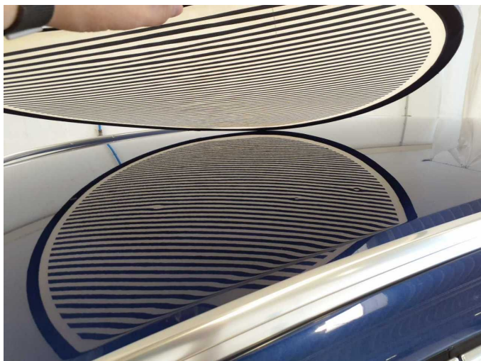
Damage 17: Body: Body - Damage by hail - Repair
