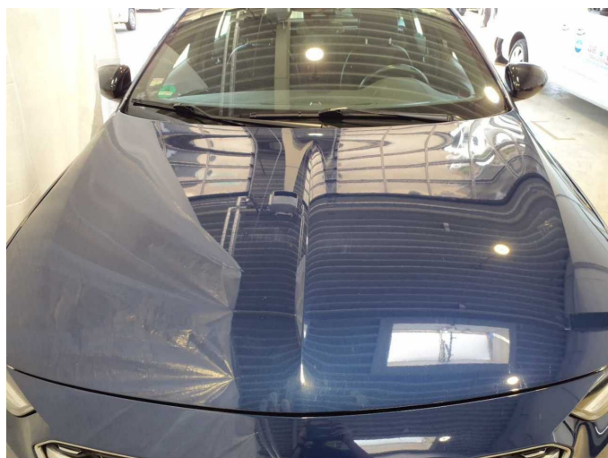
Damage 17: Body: Body - Damage by hail - Repair
