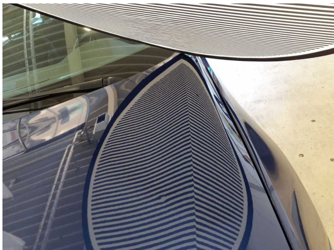
Damage 17: Body: Body - Damage by hail - Repair
