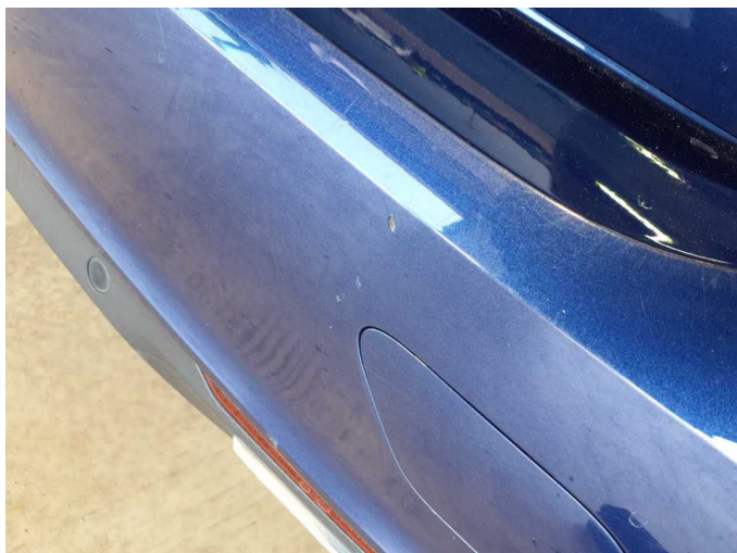
Damage 10: Rear bumper: Rear bumper - Scratch(es) - Paint
