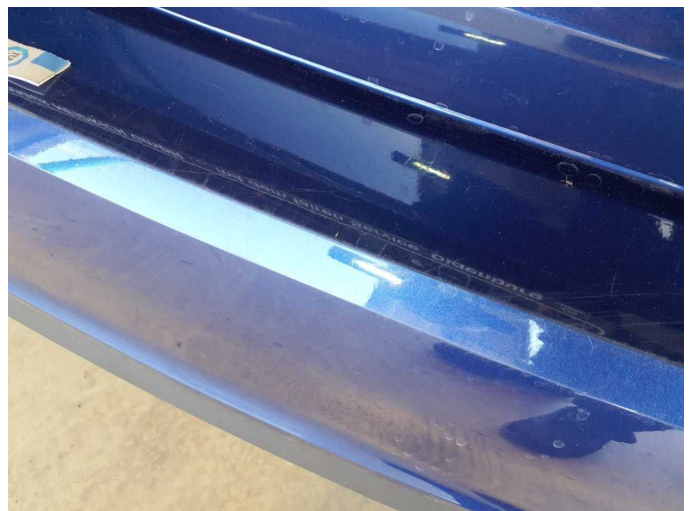
Damage 10: Rear bumper: Rear bumper - Scratch(es) - Paint
