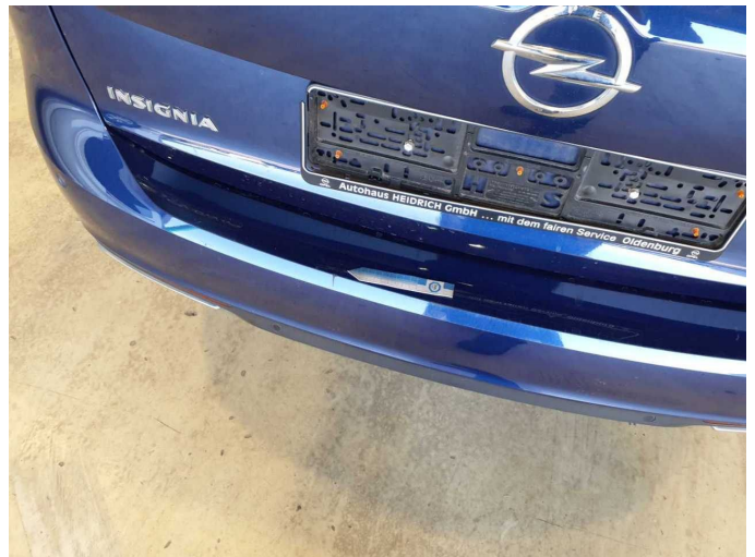
Damage 10: Rear bumper: Rear bumper - Scratch(es) - Paint
