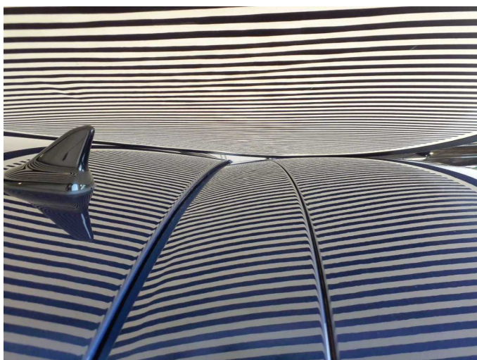
Damage 17: Body: Body - Damage by hail - Repair
