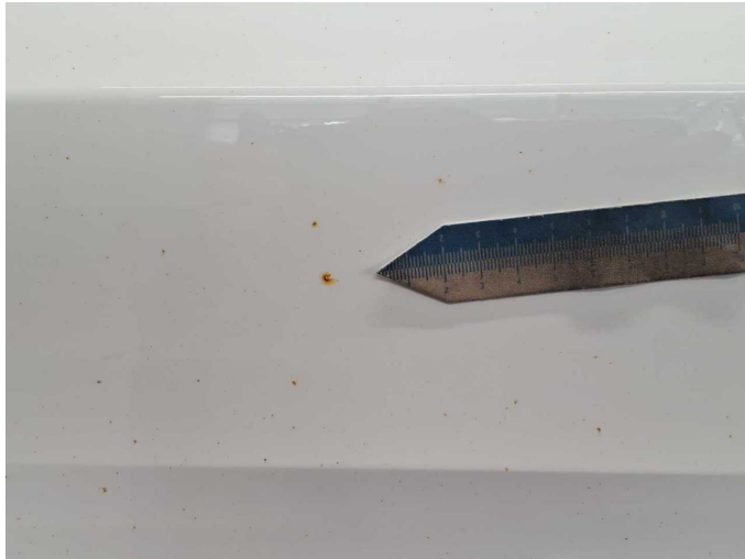
Damage 3: Body: Body (Flugrost) - Corrosion - Smart repair
