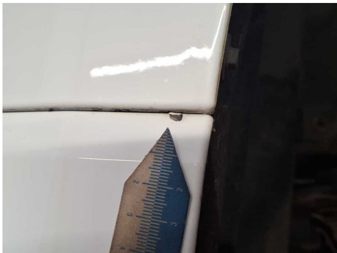
Damage 5: Rear bumper: Spoiler (Rechts) - Scratch(es) - Paint
