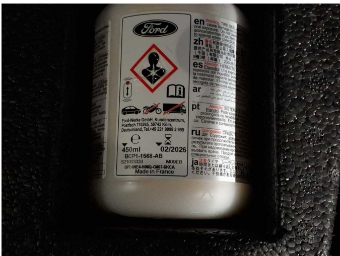
Damage 2: Equipment: Tirefit filler - Expired - Replace
