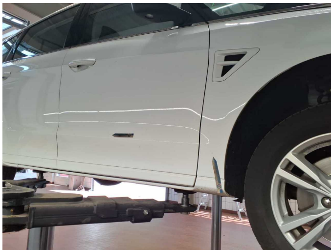
Damage 3: Body: Body (Flugrost) - Corrosion - Smart repair
