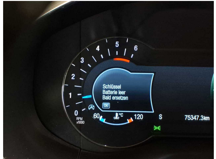
Damage 1: Equipment: Vehicle key with remote control (Batterie) - Empty - Replace
