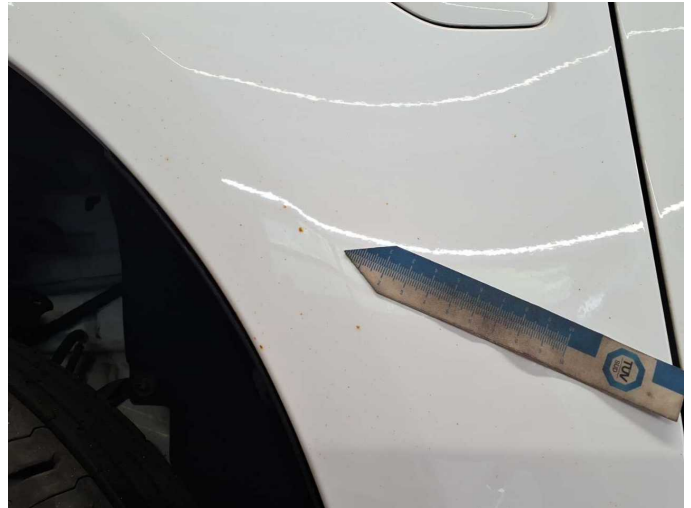
Damage 3: Body: Body (Flugrost) - Corrosion - Smart repair
