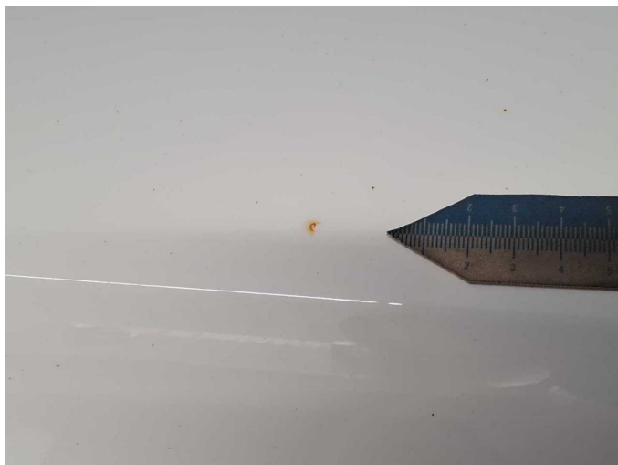
Damage 3: Body: Body (Flugrost) - Corrosion - Smart repair
