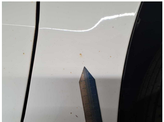
Damage 3: Body: Body (Flugrost) - Corrosion - Smart repair
