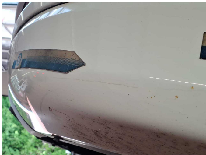
Damage 5: Rear bumper: Spoiler (Rechts) - Scratch(es) - Paint
