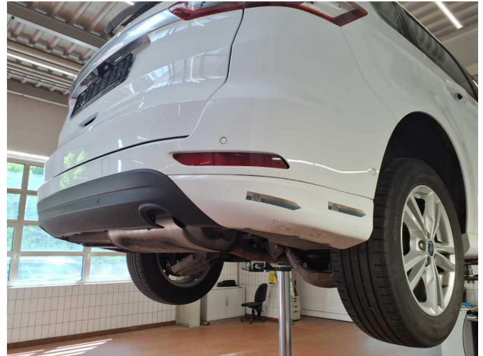
Damage 5: Rear bumper: Spoiler (Rechts) - Scratch(es) - Paint
