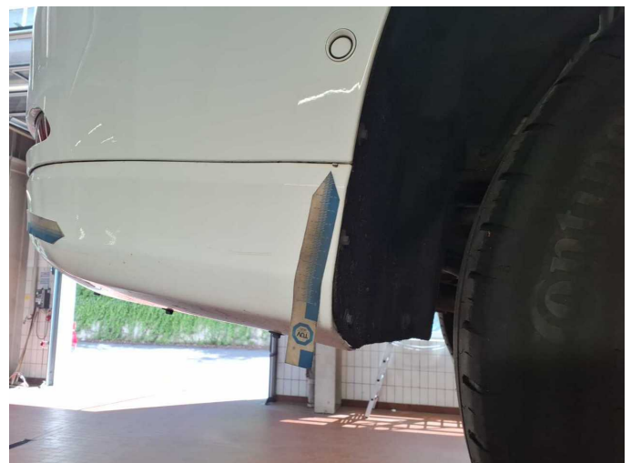
Damage 5: Rear bumper: Spoiler (Rechts) - Scratch(es) - Paint
