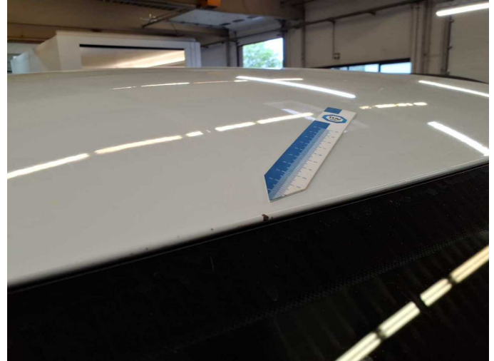
Damage 4: Roof: Roof (Randbereich) - Stone chips - Smart repair
