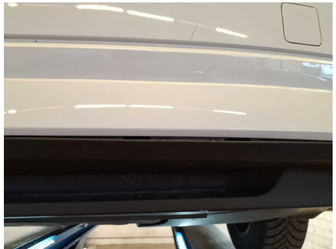
Damage 2: Rear bumper: Spoiler - Malposition - Repair
