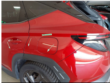
Kotflügel / Hinten Links / Delle
