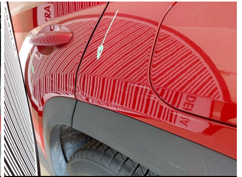
Kotflügel / Hinten Links / Delle
