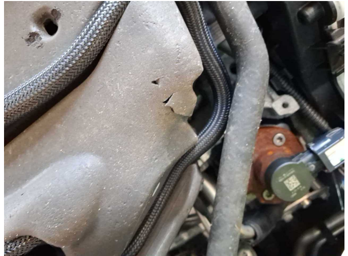
Missing part 1: Engine: Engine cover (+Maderbiss) - Missing - Replace
