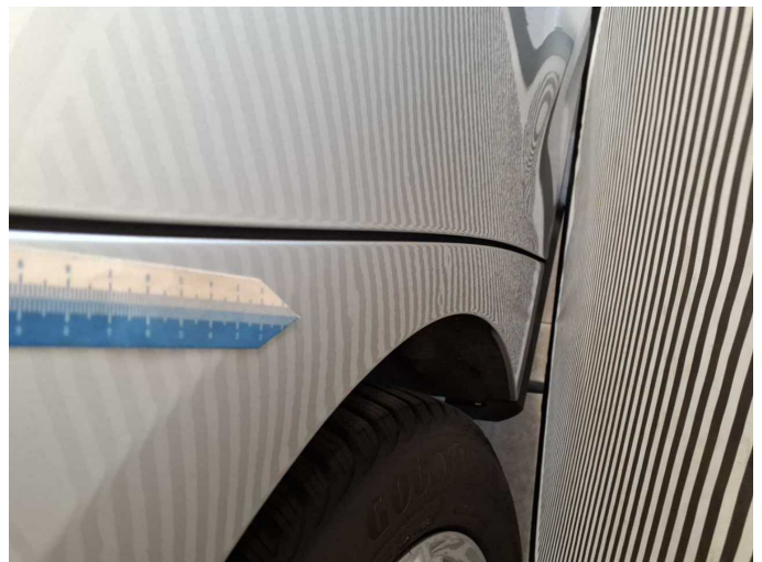
Damage 1: Side panel - rear right side: Elbow (3) - dent(s) - Smart repair
