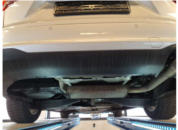
Damage 2: Rear bumper: Spoiler (Loch für anhängerkuppl. fehlt) - does not comply with manufacturer's specifications - Replace
