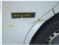
Mirror side repeater R, Scratch(es), Replace
