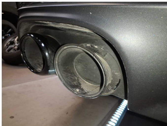
Damage 4: Exhaust system: Exhaust system (Blende) - Missing - Replace
