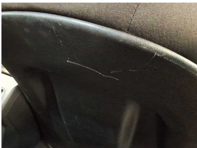
Damage 7: Seat - front: Seat - right side (Rückenlehne Schale) - Scratched - Replace
