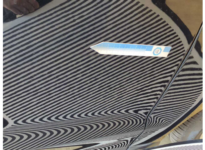
Damage 6: Door - front right side: Door (Wellig) - Unprofessionally repaired - Repair and paint
