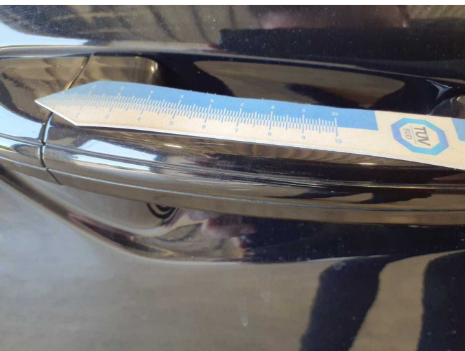
Damage 1: Door - front right side: Door handle - outside - Scratch(es) - Smart repair
