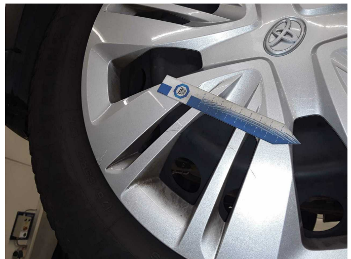
Damage 1: Wheel / tyres: Wheel cover - front left side - Scratched - Replace
