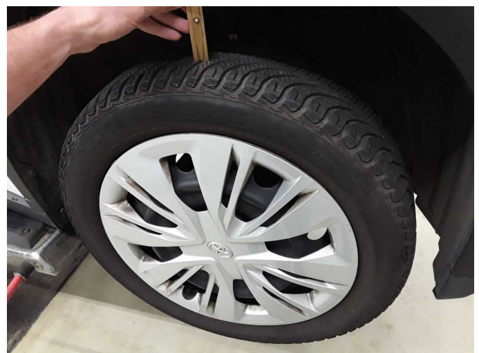
Damage 7: Wheel / tyres: Tyre - front - Does not meet the leasing specifications - Replace
