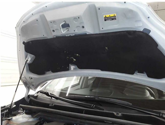
Damage 6: Bonnet: Insulation lining - Damage caused by marten / rodent - Replace
