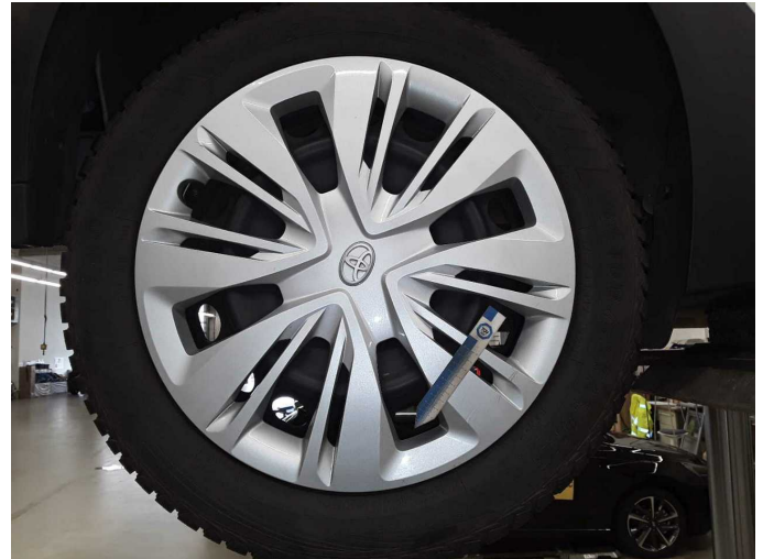
Damage 2: Wheel / tyres: Wheel cover - rear right side - Scratched - Replace
