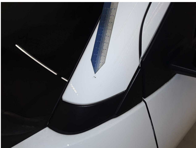
Wear and tear 1: Roof: Roof rail - left side - Stone chips - No deduction
