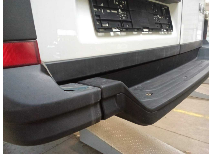
Wear and tear 2: Rear bumper: Rear bumper - Malposition - No deduction
