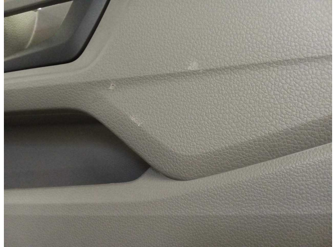
Damage 3: Trim / covers: Door trim - front right side - Scratch(es) - Smart repair
