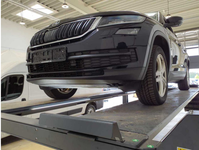
Damage 4: Front bumper: Spoiler - Deformed - Replace
