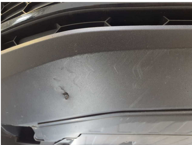
Damage 4: Front bumper: Spoiler - Deformed - Replace
