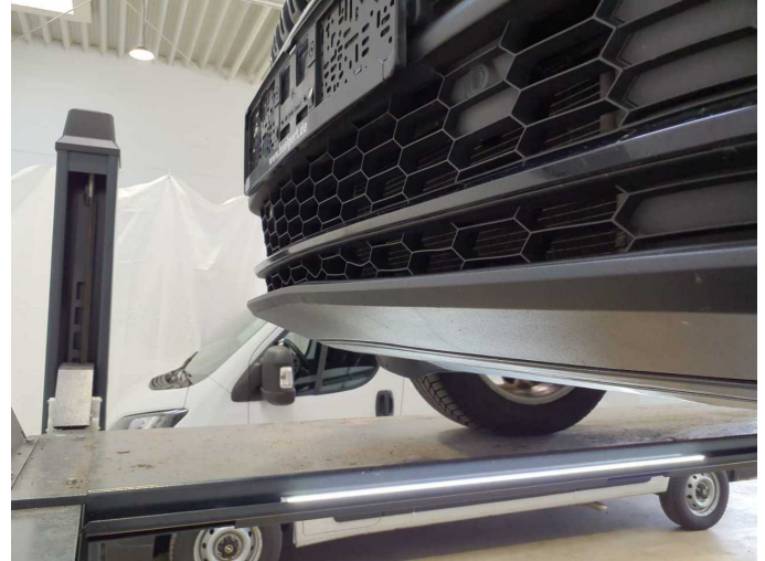
Damage 4: Front bumper: Spoiler - Deformed - Replace
