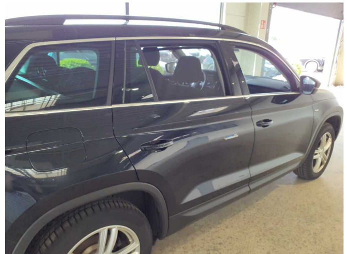
Damage 6: Door - rear right side: Door - Deformed - Repair and paint
