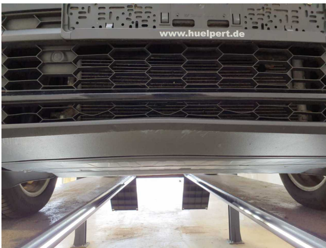
Damage 4: Front bumper: Spoiler - Deformed - Replace
