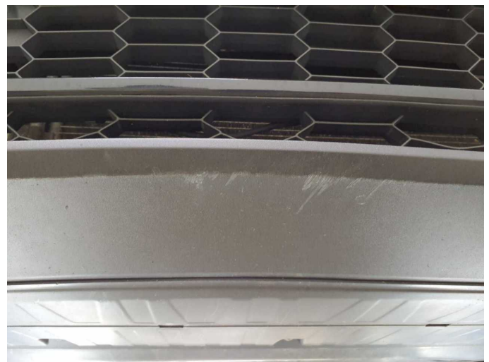
Damage 4: Front bumper: Spoiler - Deformed - Replace
