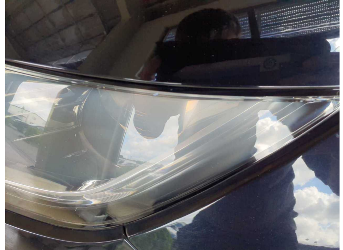
Damage 7: Headlight: Headlight - left side (+ Rechts / Milchig) - Not admissible - Replace
