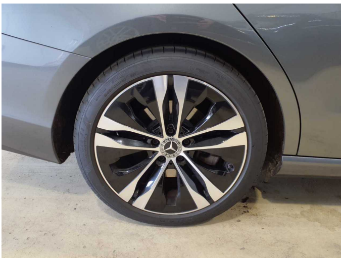
Damage 6: Wheel / tyres: Tyre - rear right side (nicht fahrbereit) - Porous / cracked - Replace
