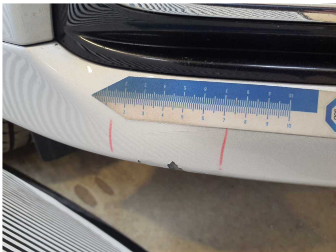
Damage 1: Front bumper: Spoiler - Scratch(es) - Smart repair
