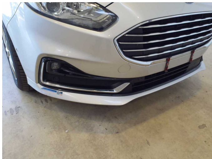
Damage 1: Front bumper: Spoiler - Scratch(es) - Smart repair
