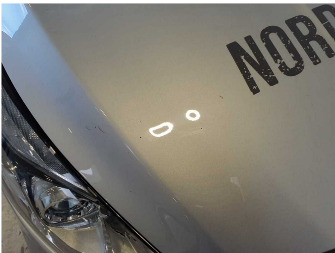
Damage 9: Bonnet: Bonnet - Stone chips - Paint
