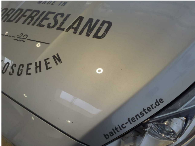
Damage 9: Bonnet: Bonnet - Stone chips - Paint
