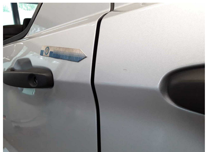
Damage 1: Sliding door - left side: Sliding door - Dent / paintcoat damage - Repair and paint
