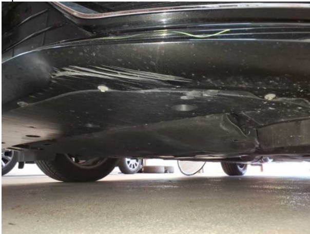
Damage #7: Front bumper: Front bumper - Scratched - Loss in value
