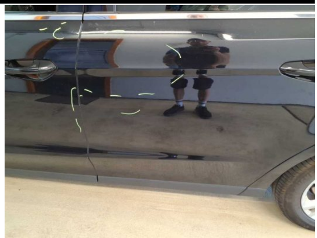
Damage #5: Door - rear left side: Door - Scratched - Cover / polish
