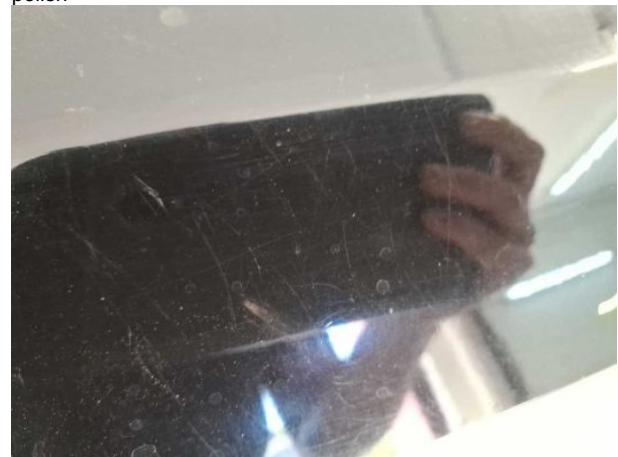
Damage #3: Boot lid / rear door: Boot lid - Scratched - Cover / polish
