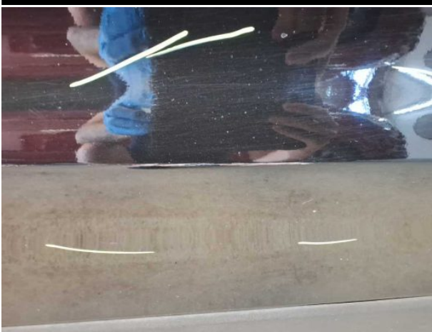
Damage #13: Door - front right side: Door - Scratched - Repair and paint
