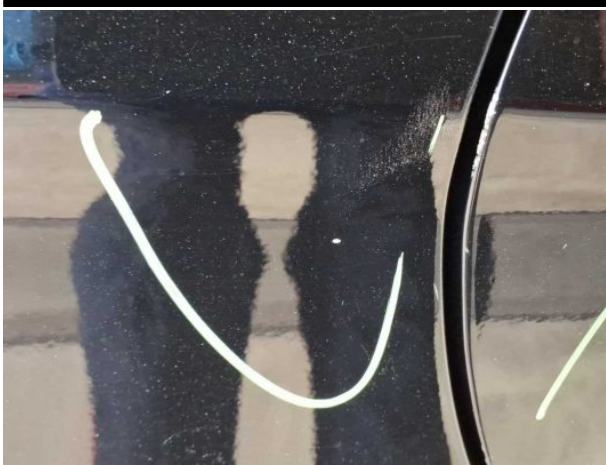
Damage #9: Side panel - rear right side: Side panel - Dent / paintcoat damage - Smart repair
