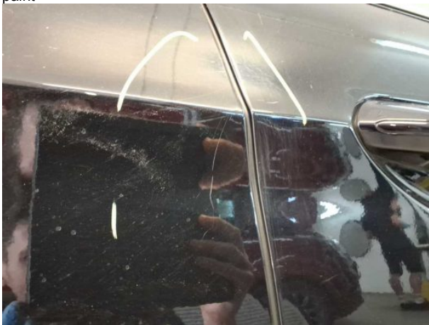
Damage #12: Door - rear right side: Door - Scratched - Repair and paint
