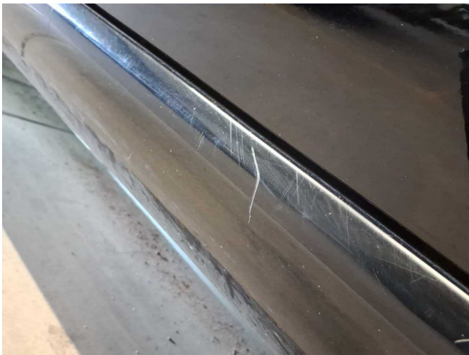
Damage 7: Sill - left side: Trim - Scratch(es) - Paint
