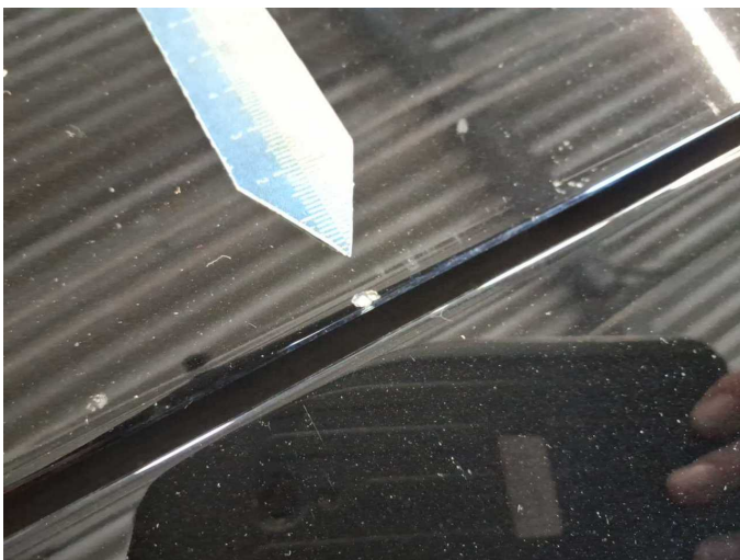
Damage 11: Bonnet: Bonnet - Stone chips - Paint
