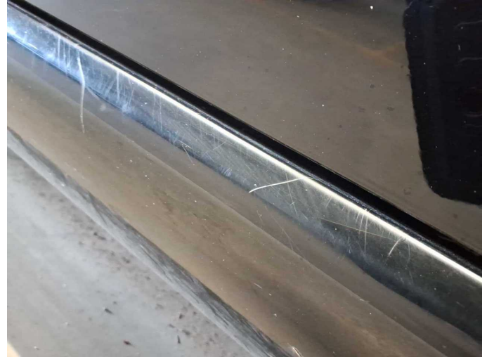
Damage 7: Sill - left side: Trim - Scratch(es) - Paint
