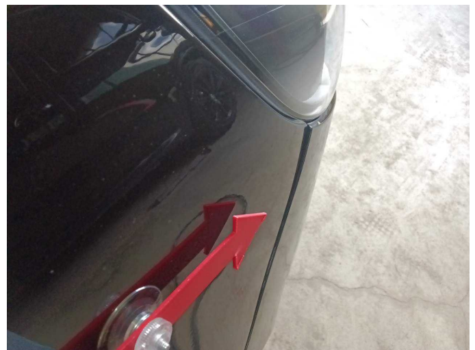
Damage 2: Front bumper: Front bumper - Malposition - Un- / install
