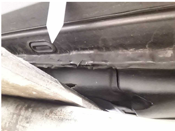
Damage 8: Sill - right side: Sill - Scratch(es) - Smart repair
