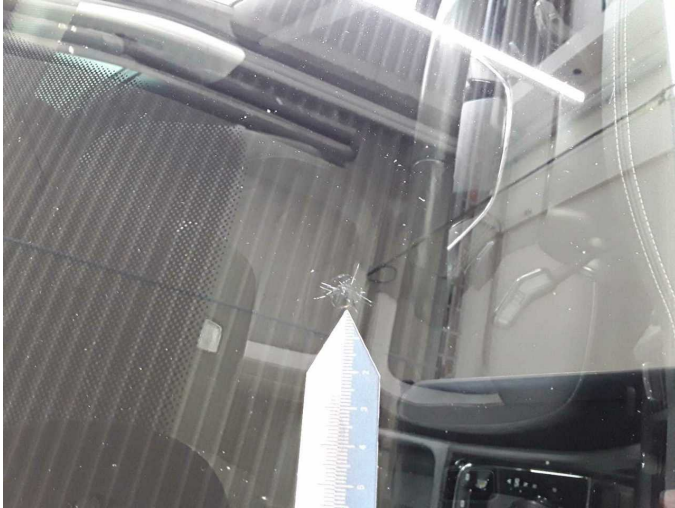
Damage 10: Vehicle glazing: Windscreen - Stone chips - Replace
