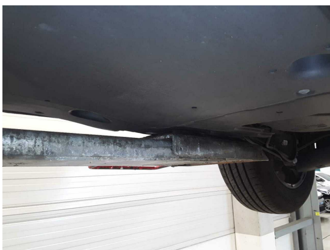
Damage 7: Body: Underbody panelling - Broken / torn - Replace
