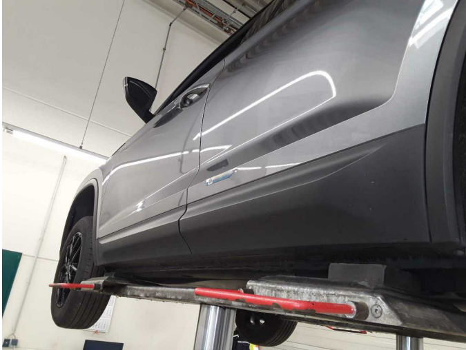
Wear and tear 3: Door - rear left side: Door - dent(s) - No deduction
