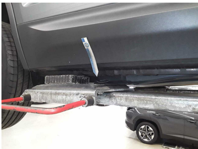
Damage 7: Body: Underbody panelling - Broken / torn - Replace
