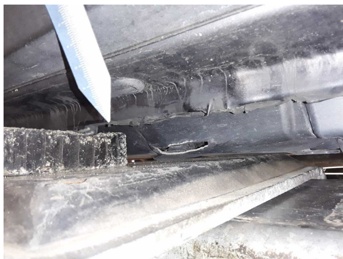
Damage 7: Body: Underbody panelling - Broken / torn - Replace
