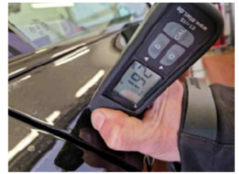
Paint thickness Door FR
