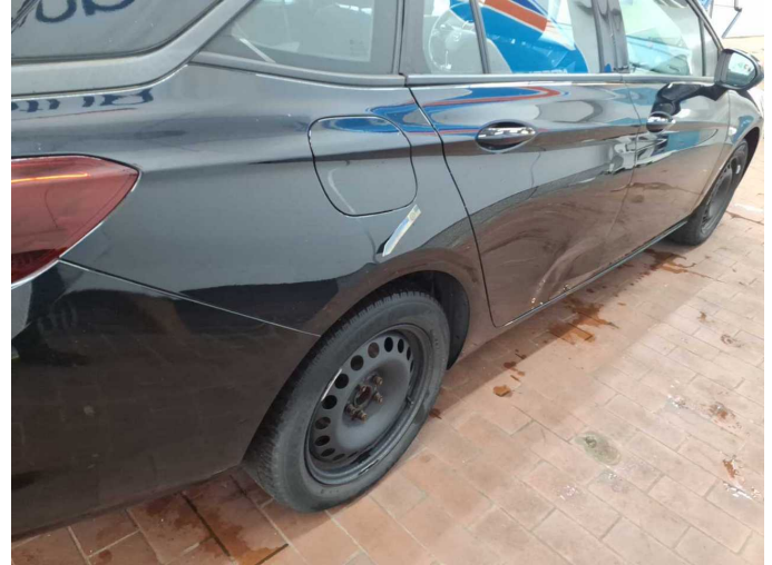
Damage 19: Side panel - rear right side: Side panel - dent(s) - Repair and paint
