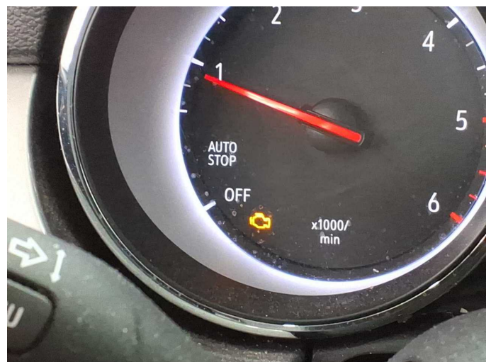
Damage 14: Instrument panel: Indicator light (Motorkontrolleuchte) - on - Perform diagnosis
