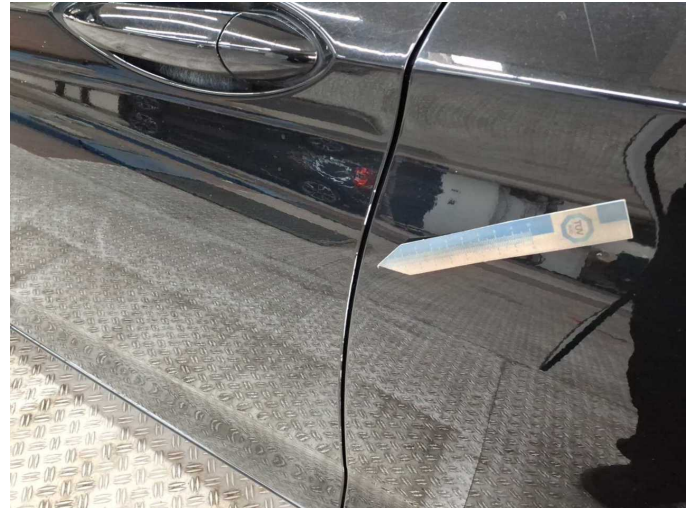
Damage 9: Door - front left side: Door edge - Scratch(es) - Smart repair
