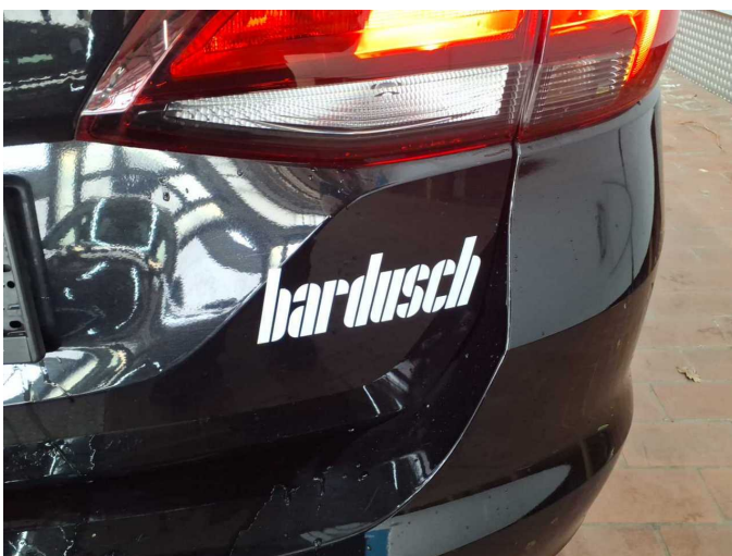
Damage 10: Boot lid / rear door: Boot lid - Glued / labelled - De-glu / neutralise
