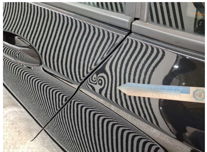
Damage 8: Side panel - rear left side: Side panel - dent(s) - Smart repair
