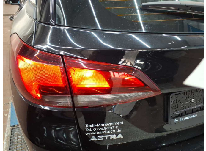
Damage 15: Tail light: Tail lamp - left side - Broken / torn - Replace
