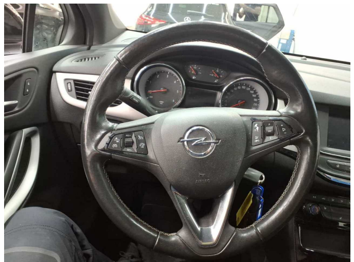
Damage 3: Steering system: Steering wheel - Abrasion - Loss in value
