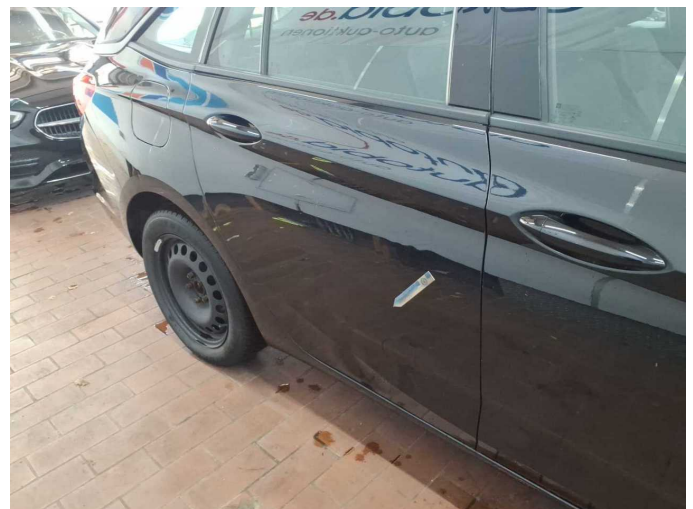
Damage 20: Door - rear right side: Door - Deformed - repair according to calculation
