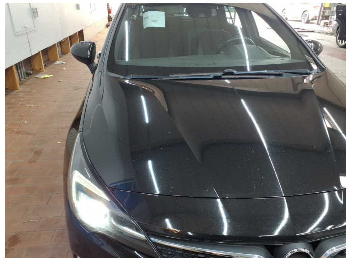
Damage 18: Bonnet: Bonnet - Stone chips - Paint
