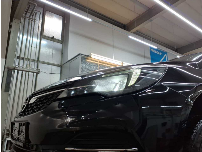
Damage 17: Headlight: Headlight - left side (Klarlack löst sich) - Paint defect - Replace
