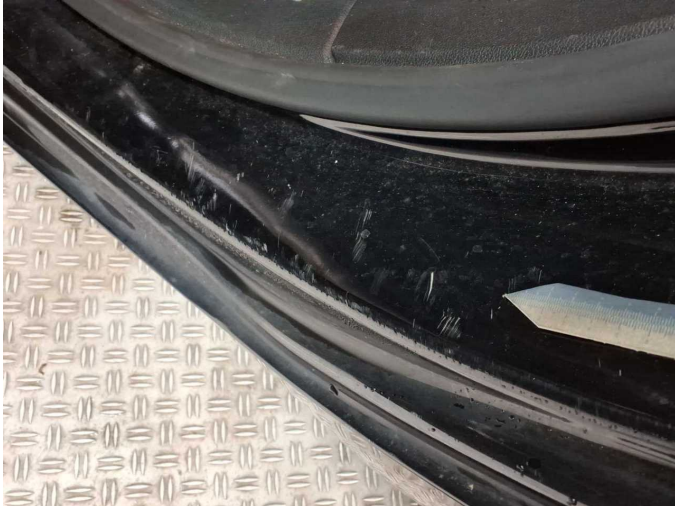
Damage 11: Side panel - rear left side: Sill - Scratch(es) - Smart repair
