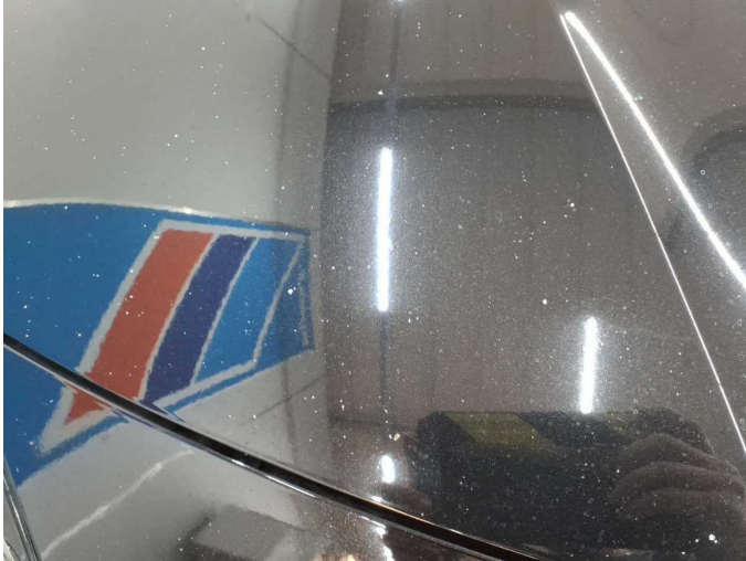
Damage 18: Bonnet: Bonnet - Stone chips - Paint
