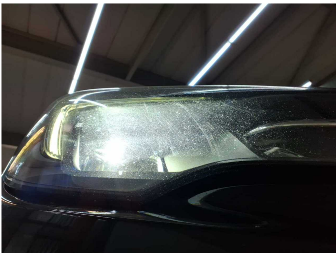
Damage 16: Headlight: Headlight - right side (Klarlack löst sich.) - Paint defect - Replace
