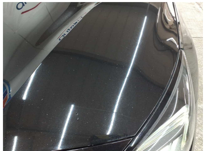
Damage 18: Bonnet: Bonnet - Stone chips - Paint
