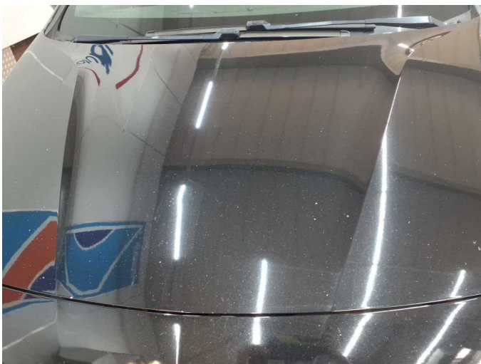
Damage 18: Bonnet: Bonnet - Stone chips - Paint
