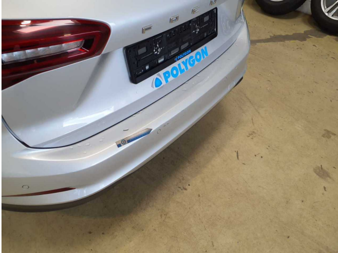
Damage 6: Rear bumper: Bumper with Parktronic - Scratch(es) - Paint
