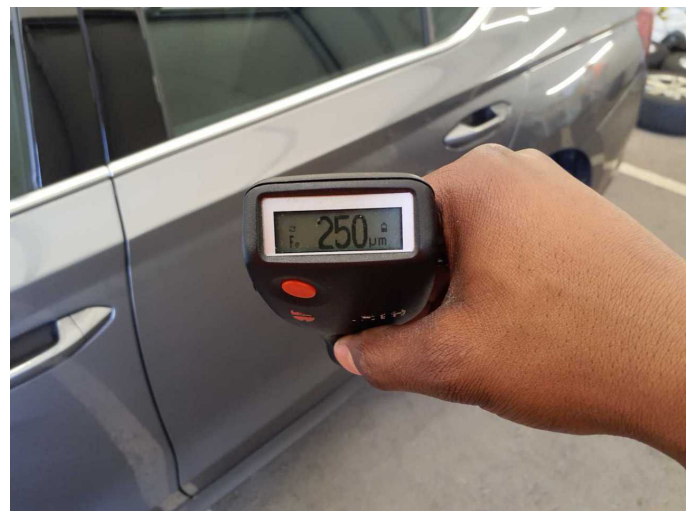
Repainting 2: Door - rear left side
