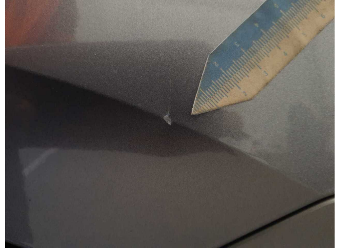
Damage 3: Side panel - rear left side: Side panel - Dent / paintcoat damage - Smart repair
