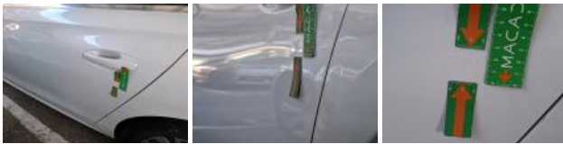
Wing RL, Dent(s), Repair and paint (complete)
