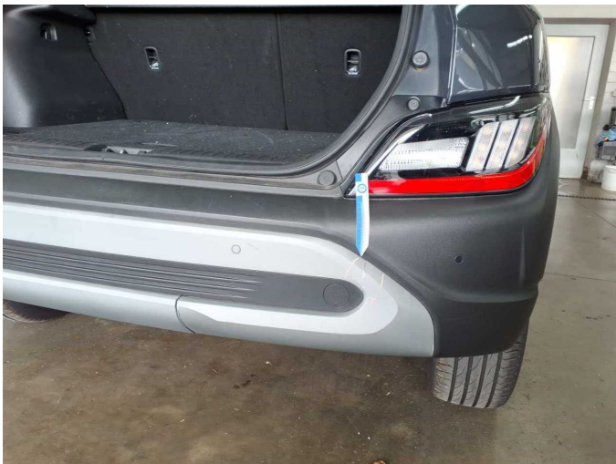
Damage 12: Rear bumper: Rear bumper (Gestaucht + Spoiler gebrochen erneuern) - Deformed - Replace
