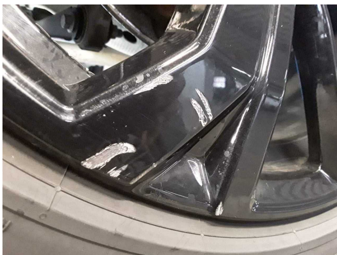
Damage 3: Wheel / tyres: Alloy rim - rear left side (Materialabtrag) - Scratch(es) - Loss in value
