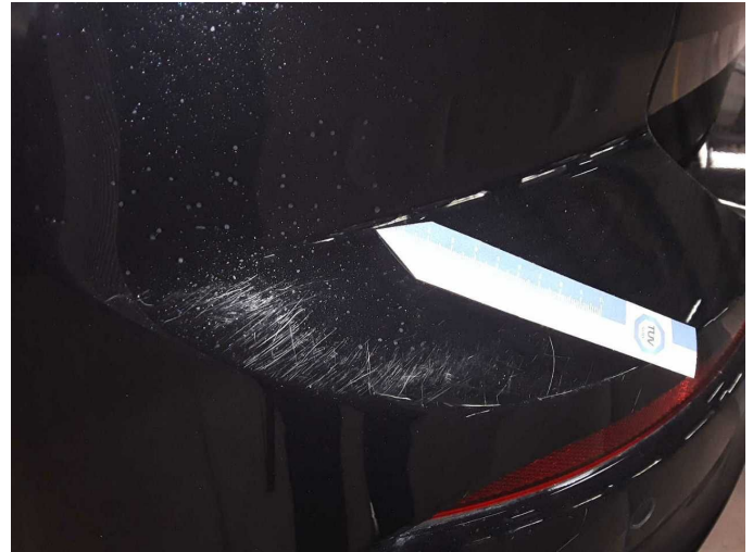
Damage 6: Rear bumper: Rear bumper - Scratch(es) - Paint
