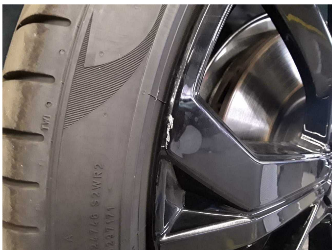
Damage 2: Wheel / tyres: Alloy rim - front right side - Scratch(es) - Smart repair
