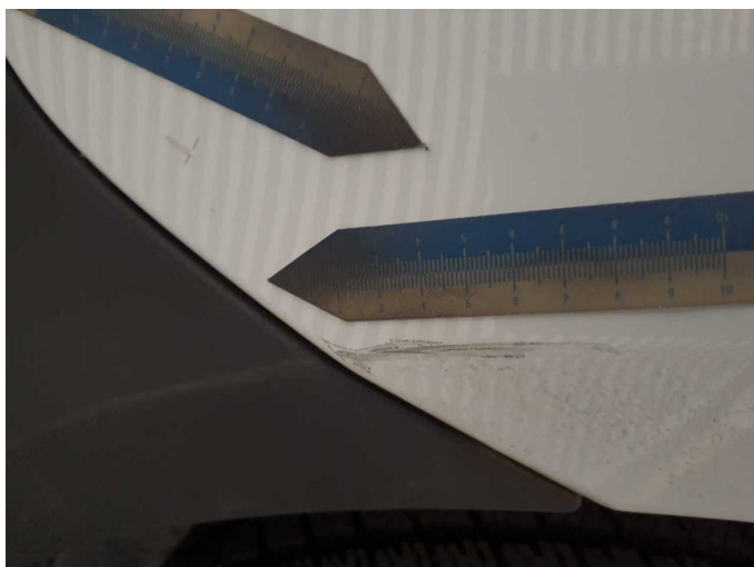
Damage 6: Mudguard - left side: Mudguard - left side - Scratch(es) - Paint
