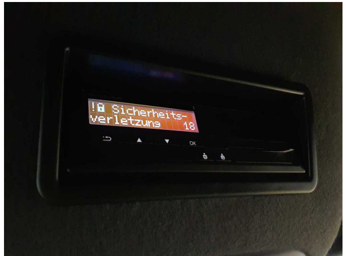
Damage 5: Misc.: Tachograph inspection (Sicherheitsverletzung) - Functional / admissibility - Perform diagnosis
