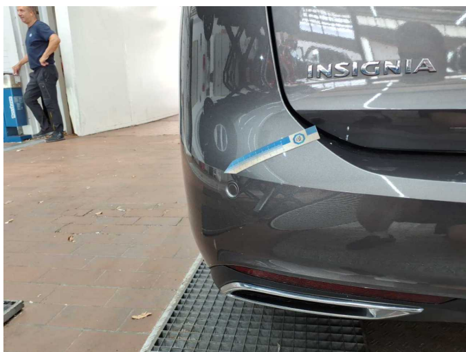
Damage 10: Rear bumper: Rear bumper - Scratch(es) - Paint
