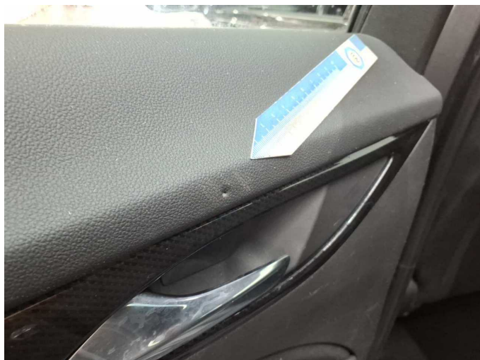
Damage 2: Trim / covers: Door trim - rear left side - Deformed - Loss in value
