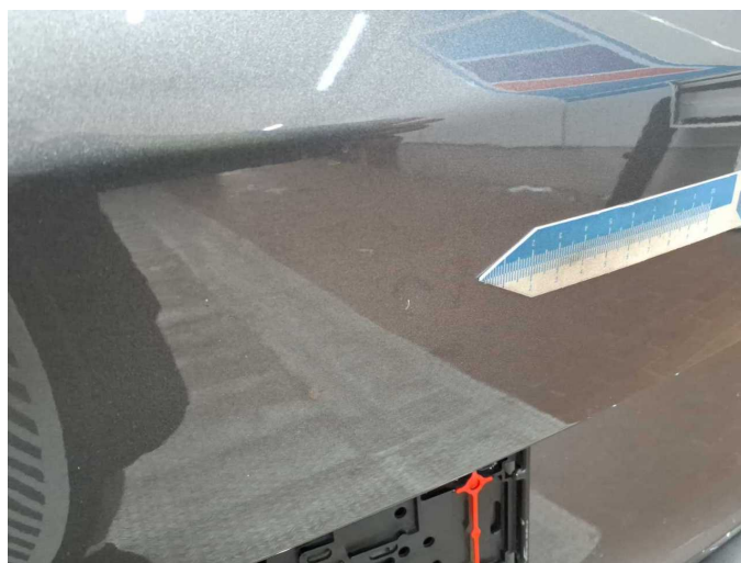
Damage 4: Boot lid / rear door: Boot lid - Dent / paintcoat damage - Smart repair
