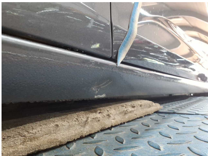
Damage 7: Sill - left side: Sill - Dent / paintcoat damage - Smart repair
