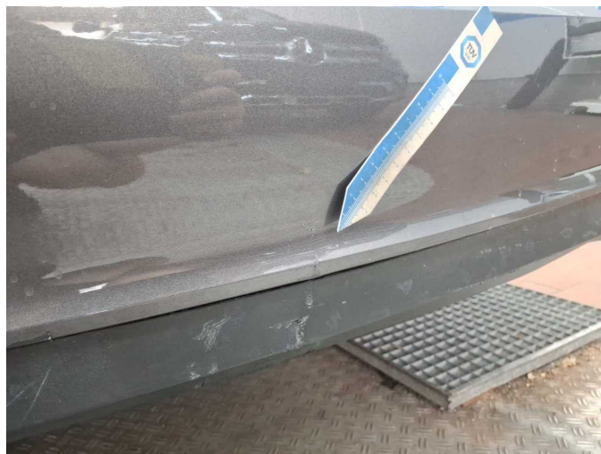
Damage 10: Rear bumper: Rear bumper - Scratch(es) - Paint
