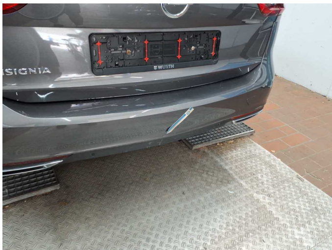
Damage 10: Rear bumper: Rear bumper - Scratch(es) - Paint
