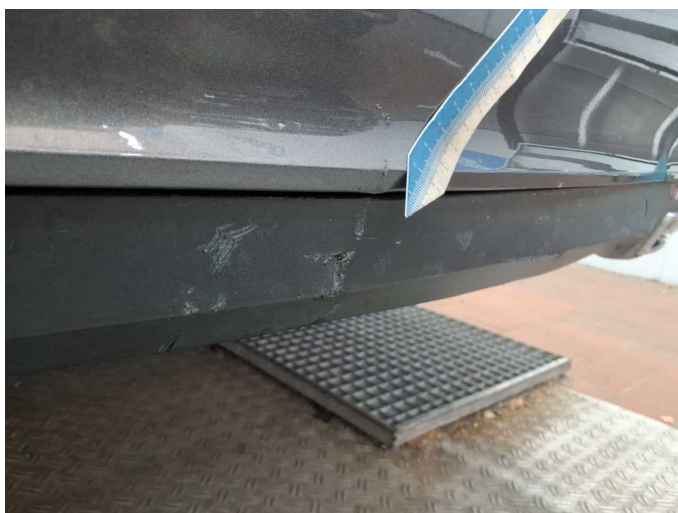
Damage 8: Rear bumper: Spoiler - Deformed - Replace
