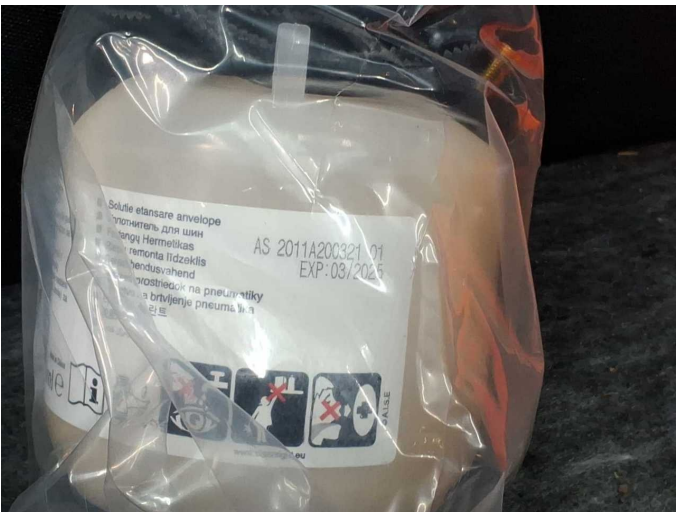
Damage 1: Equipment: Tirefit filler - Expired - Replace
