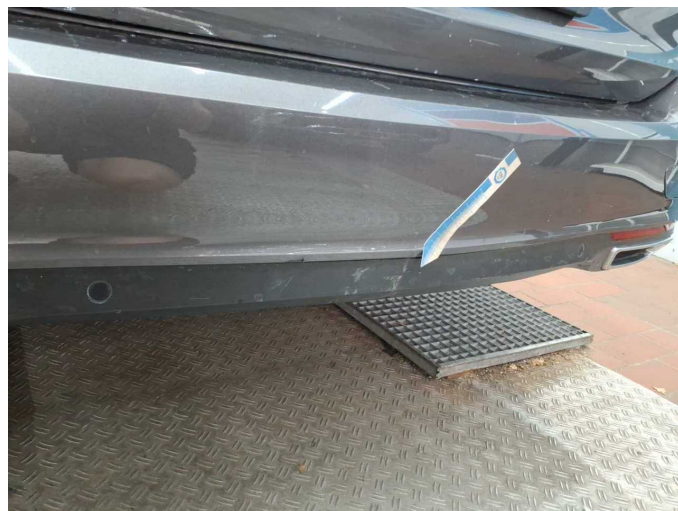
Damage 8: Rear bumper: Spoiler - Deformed - Replace
