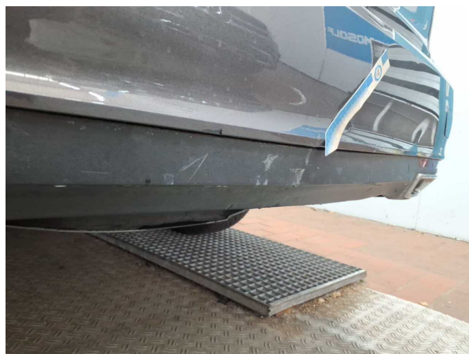
Damage 8: Rear bumper: Spoiler - Deformed - Replace
