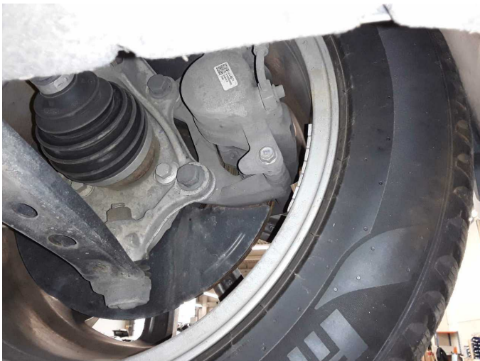
Damage 8: Braking system: Brake discs and brake pads - front (Verschlissen und) - Corrosion - Replace
