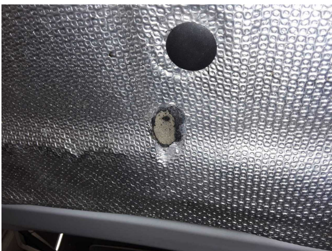
Damage 4: Bonnet: Insulation lining - Broken / torn - Replace
