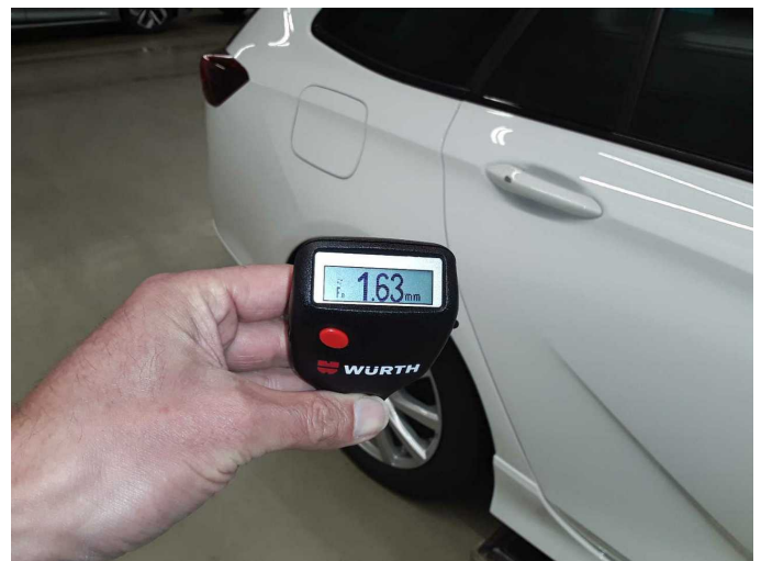
Side panel - rear right side: 1,630 µm
