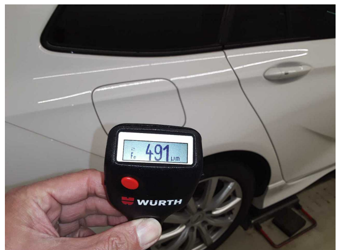
Repainting 1: Roof, Side panel - rear right side, Door - rear left side, Door - rear right side, Door - front right side
