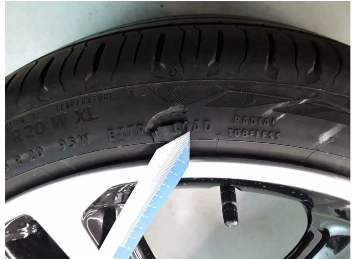
Damage 3: 2nd wheel set: 1 tyre - Broken / torn - Replace
