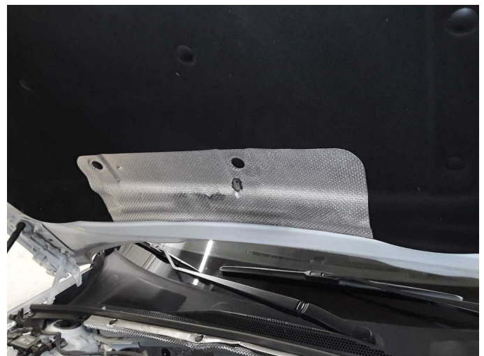
Damage 4: Bonnet: Insulation lining - Broken / torn - Replace
