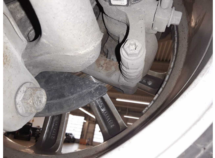
Damage 5: Braking system: Brake discs and pads - rear - Worn - Replace
