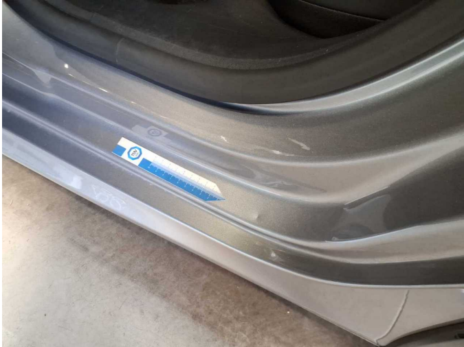
Damage 1: Side panel - rear left side: Sill - dent(s) - Smart repair
