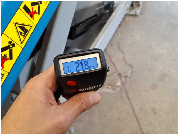
Repainting 1: Side panel - rear right side, Door - rear right side, Door - front left side, Door - front right side
