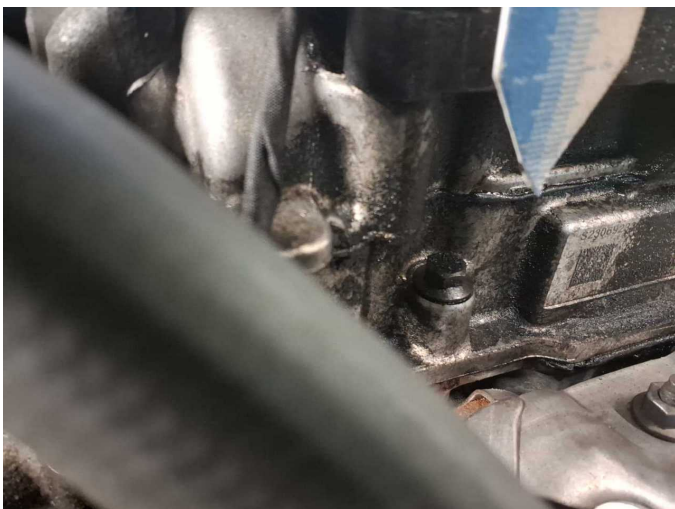
Damage 3: Engine: Engine (Ölverlust) - Leaking - Perform diagnosis
