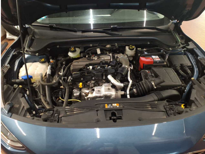
Missing part 1: Engine: Engine cover - Missing - Replace
