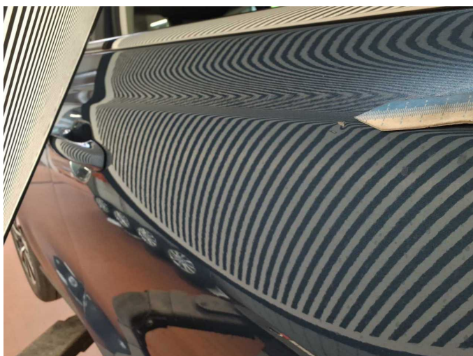
Damage 5: Door - front right side: Door - Dent / paintcoat damage - Smart repair
