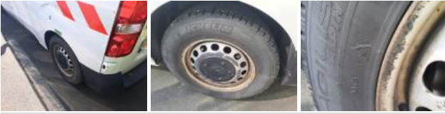
Tyre FR, Out of tolerance, Replace
