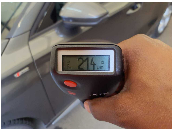
Repainting 2: Door - front left side
