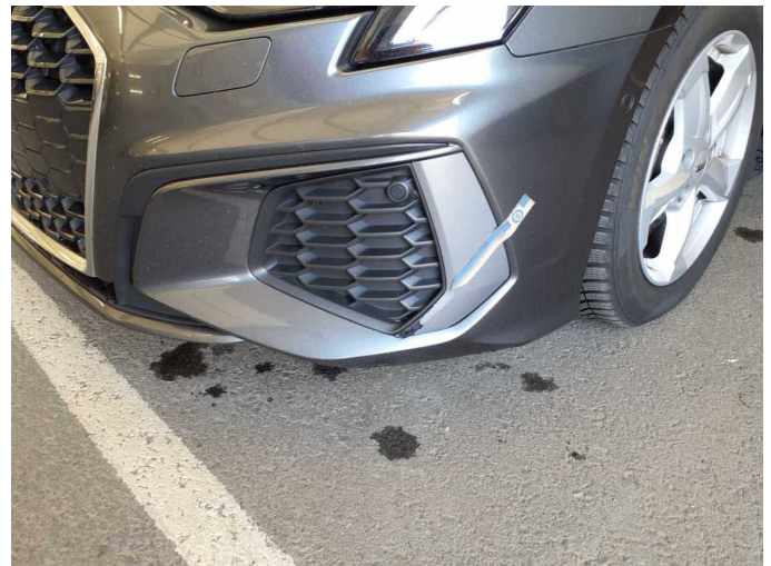
Damage 4: Trim / covers: Brightware / decorative strip (L + R) - Paint defect - Paint
