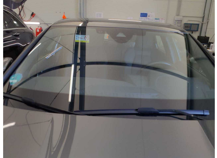
Damage 3: Vehicle glazing: Windscreen with lane departure assistant - Stone chips - Replace
